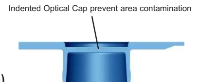
Indented Optical Cap prevent area contamination
